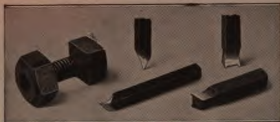
By Selecting Carefully the Kinds of Wood to be Used, and Grinding the Tools to Appropriate Shapes, Good Accurate Wood Threads can be Cut
